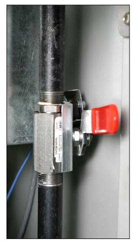
The oil discharge valve handle is shown in the OFF position. Push it down to discharge oil from the filter pan.
