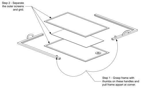
2. Separate the outer screens and grid.
